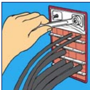
1 Remove the nuts and the hardware from the face of the endpacking.
