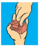
Select a suitable standard Block or AddBlock for the small cable. Then create a base using U-Blocks. The external measurements should be the same as the previous block.
