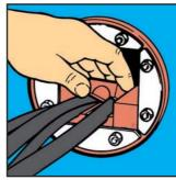
Tighten the bolts to compress and complete the seal.
