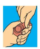
Place the plug in the AddBlock and make sure the locking devices secure it in place.
