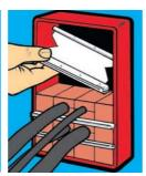
3 Begin packing. A stayplate is inserted between each layer of insert blocks.
